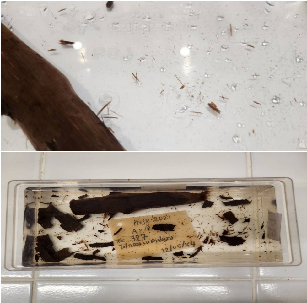
Figure 9. Degradation behavior of wood during desalination process.
